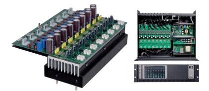
The POW2 is a sixteen channel power amplifier kit which is an optional device to be installed inside the R2 Multi-Zone and M2 Multi-Media Digital Matrix systems.
