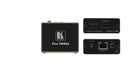
PT-872xr is a high-performance, long-reach DGKat<sup>™</sup> 2.0 receiver for 4K@60Hz (4:4:4) HDR HDMI and HDCP 2.2 signals and 2-way powering over twisted pair. It converts the transmitted DGKat<sup>™</sup> 2.0 signal into an HDMI signal. PT-872xr extends the signal to up to 60m (200ft) at 4K@60Hz (4:4:4) resolution and up to 70m (230ft) at 4K@30Hz (4:4:4) 24bpp resolution over Kramer shielded cables
