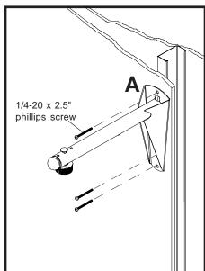
Attach wall arm with 1/4-20 phillips screws.
