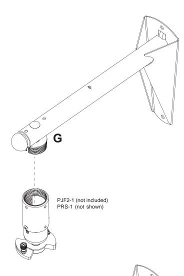
Secure PJF2-1 to threaded rod adapter (G) with one #10-32 x 3/8 socket pin screw provided with PJF2-1
