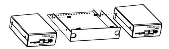
2. Connect the short side plates, one on each side of the rack.
