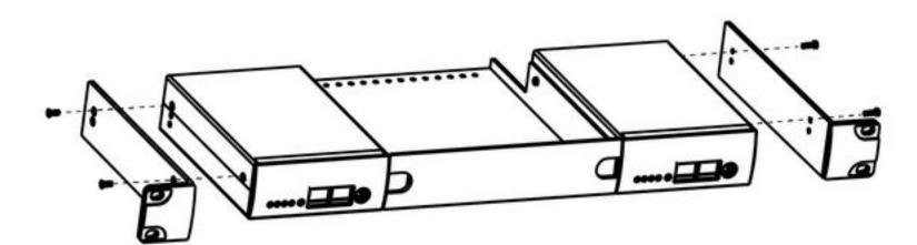
Once assembled and secured, rack mount it using the provided mounting screws and washers.
