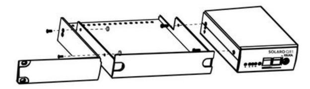
3. Connect the short side plate to the end of the Solaro device.
