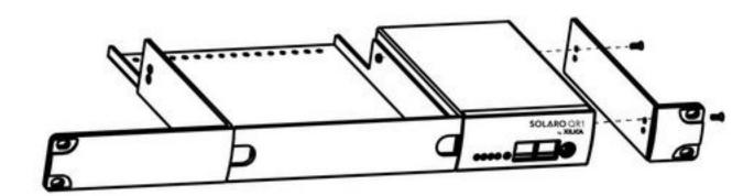
4. Once assembled and secured, rack mount it using the provided mounting screws and washers. You can use the center piece to store power supplies and cables. The holes in the centre piece are for cable ties.
