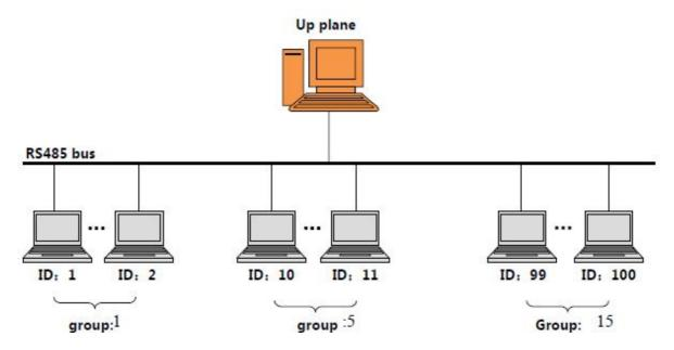
Note: This version of the protocol support the maximum number of terminal devices of 1,000 units, the most can be divided into 16 groups. Serial port parameters: Baud Rate 4800bps, data bit 8, stop bit 1, no parity, no flow control.
