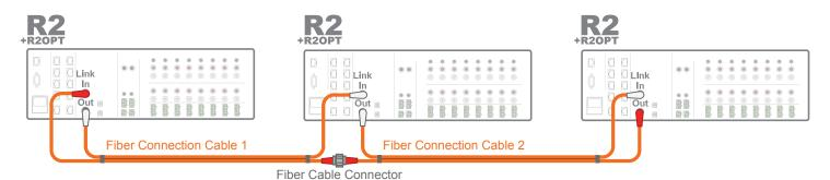
Multiple R2 units follow the same principle as with two R2 units. Each R2 has a fiber **input** and a fiber **output**. **the first device's link output is connected to the second device's link input**. Then the second's output to the third's input etc. **The final fiber out is then connected to the very first device's optical link input**, using the second available fiber cable in the dual fiber connection cable. Multiple cables need to be connected using fiber cable couplers.
