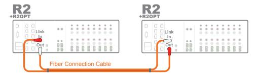
Each R2 has a fiber **input** and a fiber **output**, the connection is always done in a ring, **linking the first device's optical link output with the second device's optical link input** and vice versa. The maximum distance that can be covered is 1000m. Repeaters can be used if longer distances need to be covered.
