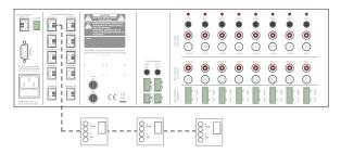
Multiple DW3020/4020 Wall panels on one PI Port (PI1 to PI10)
