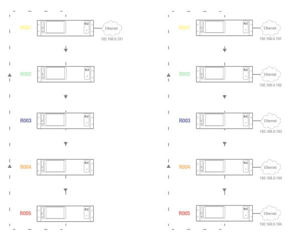
Example setup with 5 R2's, on the left side with only one Ethernet connection (Method 1) while on the right side every R2 has a separate ethernet connection (Method 2)
