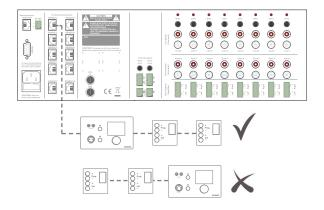
Multiple DW3020/4020 and one DW5066 Wall panel on one PI Port (PI1 to PI8) Connecting one or multiple DW3020/4020 in front of the DW5066 wall panel will cause problems.
