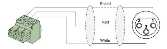
For unbalanced line in, output & priority connections:
