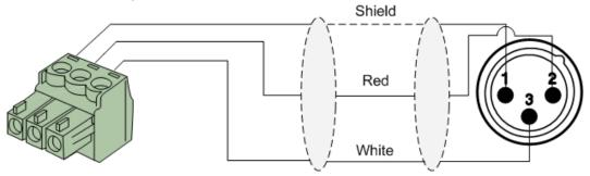
For balanced line output connections:
