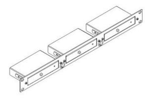
19-inch rack adapter for mounting 3 Kramer TOOLS<sup>™</sup> into a 1U rack space
