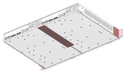
**Underside of Two SLX300s Prepared for Front Attachment Rack Mount with Joiner Plate**
