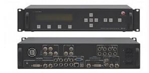
The SP-14 is a broadcast grade MEMC frame rate/standards converter. It accepts HD, SD & computer graphics signals, performs frame rate conversion, format conversion, frame synchronization, scan conversion and aspect ratio conversion as required, as well as embedded timecode processing and closed caption conversion. It is also applies powerful noise reduction & image enhancement to improve poor quality video
