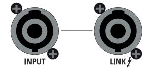
**LINK** - Power output in parallel with the INPUT socket for connecting the unit to another speaker. The number of SW2100P cabinets that can be connected in parallel depends on the amplifier load capacity.
