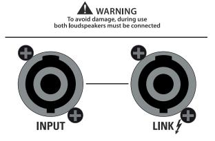
LINK - Power output in parallel with the INPUT socket for connecting the unit to another speaker. The number of SW210P cabinets that can be connected in parallel depends on the amplifier load capacity.
