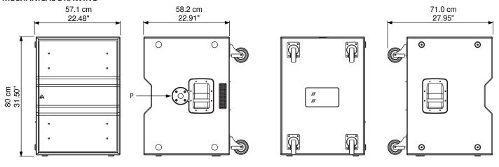
P = M20 insert for DHSS10M20 pole adaptor for conventional SUB-SAT system.
