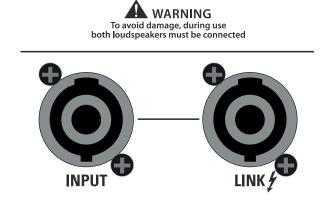
**LINK** - Power output in parallel with the INPUT socket for connecting the unit to another speaker. The number of SW215P cabinets that can be connected in parallel depends on the amplifier load capacity.
