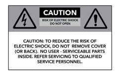
The lightning flash with arrowhead symbol, within an equilateral triangle, is intended to alert the user to the presence of uninsulated "dangerous voltage" within the product's enclosure that may be of sufficient magnitude to constitute a risk to persons.
