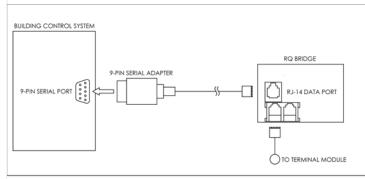
FIGURE 4: RQ BRIDGE CONNECTION TO BUILDING CONTROL SYSTEM
