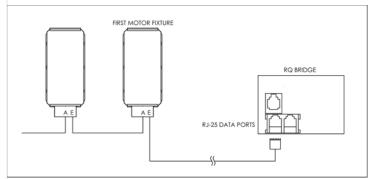
FIGURE 3: RQ BRIDGE CONNECTION TO TERMINAL MODULE
