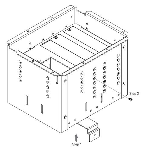
Figure 2: Installing the T-TBLANK TOOL Blank
