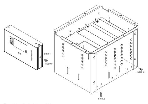
Figure 2: Installing the Kramer TOOL
