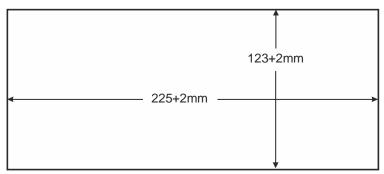
Figure 4: Cut out Dimensions
