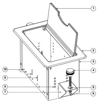
Figure 2: TBUS-4xl Enclosure Top View
