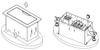
Figure 5: Inserting TBUS-4xl into the Prepared Opening
