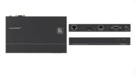
TP-581T is a high-performance, extended-reach HDBaseT transmitter for 1080p60Hz HDMI, Ethernet, RS-232 and IR signals over twisted pair. The TP-581T converts all input signals into the transmitted HDBaseT signal. It extends video signals to up to 130m (430ft) over CAT copper cables at up to 1080p@60Hz 36bpp video resolution. The TP-582R converts the HDBaseT twisted pair signal back to Ethernet, RS-232, IR and two HDMI outputs, and de-embeds the audio to S/PDIF and TOSLINK® audio outputs
