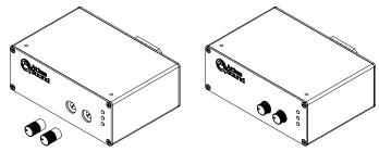
Security Cover Installation - Remove the knob from the panel and insert the cover. Small pliers may be required to remove the knobs. Align the security cover to the level control panel hole. Push the cover into the hole until it snaps into place. Do not force or damage may occur to the potentiometer.
