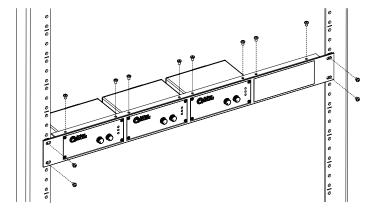
TSD-RMKHR Half Width Rack Mount Kit - Atlas Sound offers an optional rack mount kit that can
