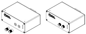
2. Security Cover Installation - Remove the knob from the panel and insert the cover. Small pliers may be required to remove the knobs. Align the security cover to the level control panel hole. Push the cover into the hole until it snaps into place. Do not force or damage may occur to the potentiometer.
