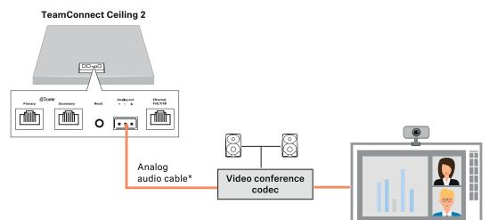
Variant 3: output analog audio signal from multiple ceiling microphones to a single DSP.
