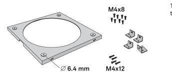
To mount the product directly below the ceiling, you need the **SL CM FB** ceiling mounting frame.
