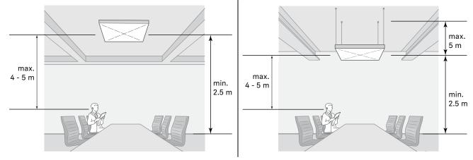
The recommended maximum distance from the speaker to the TeamConnect Ceiling 2 is 4 to 5 m. The minimum distance from the TeamConnect Ceiling 2 to the floor is 2.50 m.
