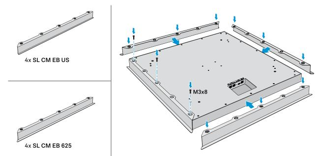
$\triangleright$  Attach the angle brackets to the TeamConnect Ceiling 2 as shown in the figure.
