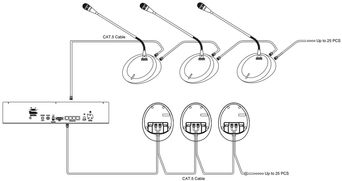
1.1 There are 4 microphone links in the back of main control unit, which can be connected randomly.
