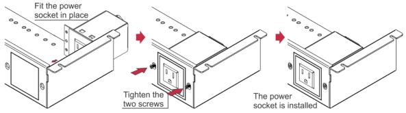
Figure 3: Installing the Power Socket
