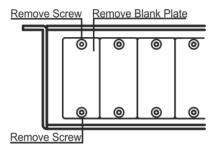
2. Place the required wall plate insert item over the opening.
