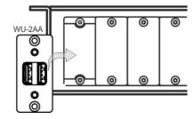
3. Reinsert the two screws to affix the wall plate insert in position and tighten them.
