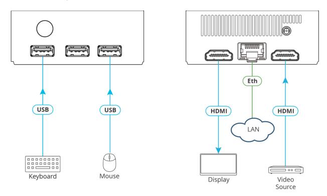
Figure 5: Connecting VIA Connect<sup>2</sup>
