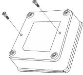
2. Fasten two screws to the bottom of VIA Connect<sup>2</sup>.
