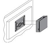
3. Insert the screws on the bottom of VIA Connect<sup>2</sup> into the slots on the mounting bracket.
