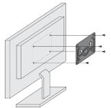
1. Attach the VESA mounting bracket to the back of the display with 4 screws.
