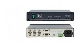
The VP-100A is a high-performance format converter for computer graphics video and stereo audio signals. It converts a computer graphics video signal on a 15-pin HD connector to an RGBHV video signal on BNC connectors and unbalanced stereo on a 3.5mm connector to balanced stereo audio on a terminal block connector.
