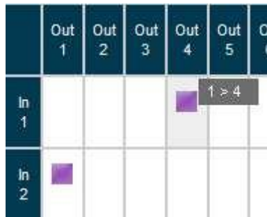
Figure 16: Switching an Input to an Output
