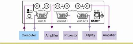
Always use Kramer high-performance cables for connecting AV equipment to the VP-2K.
