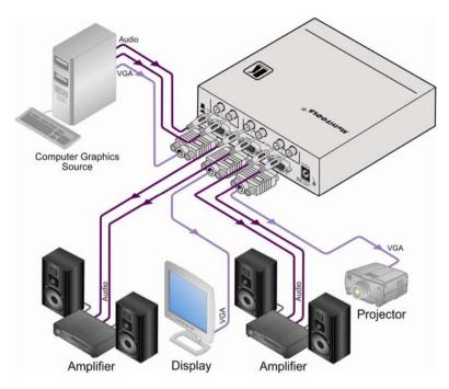
Figure 2: Connecting the VP-2K 1:2 UXGA/Audio Distributor
