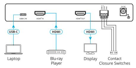
Figure 8: Connecting to the VP-424C Rear Panel
