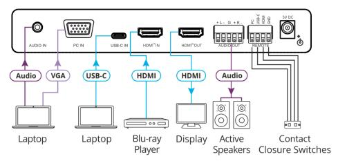
Figure 5: Connecting to the VP-426C Rear Panel
