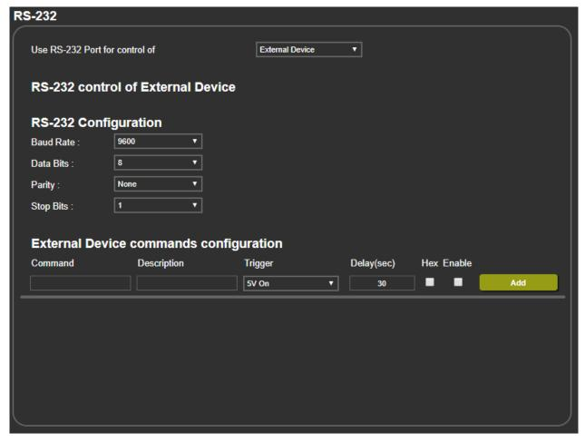
Figure 27: RS-232 Page - Controlling an External Device
