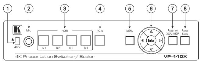
Figure 1: VP-440X 4K Presentation Switcher / Scaler Front Panel
