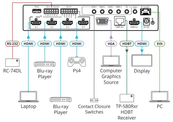
Figure 3: Connecting to the VP-440X Rear Panel
