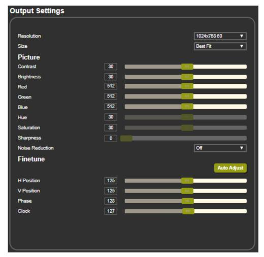
Figure 20: The Output Settings Page – PC IN is the Input
