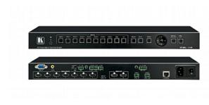
VP-550X is a versatile, professional presentation scaler/switcher for 4K@60 (4:4:4) HDMI, USB-C, VGA, and composite video signals. The unit scales the video and provides options to use the embedded digital audio or to select analog audio input signals. After processing and scaling, the embedded AV signal is sent to the 2 mirrored HDMI outputs simultaneously, and the audio is also sent to a balanced stereo audio output
