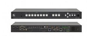
The VP-773A is a high-performance presentation switcher and scaler. It accepts one of eight inputs: one DisplayPort (DP), one composite video, two computer graphics and four HDMI signals. It scales the video, embeds the audio, and simultaneously outputs the signal to two identical HDMI and one HDBaseT TP output, together with S/PDIF and balanced stereo audio outputs. The unit also includes an audio amplifier and speaker outputs
