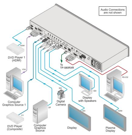
Figure 4: Connecting the VP-774 Presentation Switcher/Scaler
