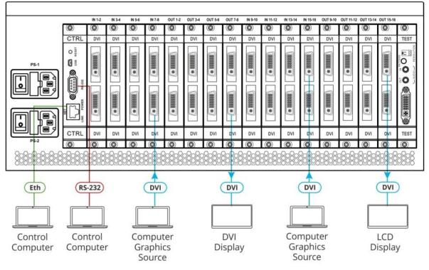
Figure 4: Connecting the VS-1616DN-EM
