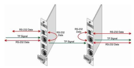
Figure 14: DGKat Card Serial Data Transmission
