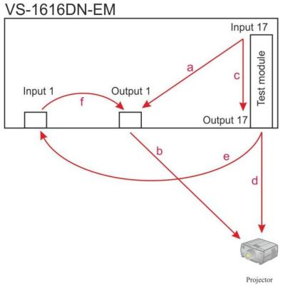
Figure 16: Signal Paths for Isolating Video Problems
