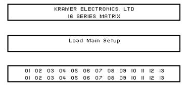
Figure 11: Default Startup Status Display Sequence
