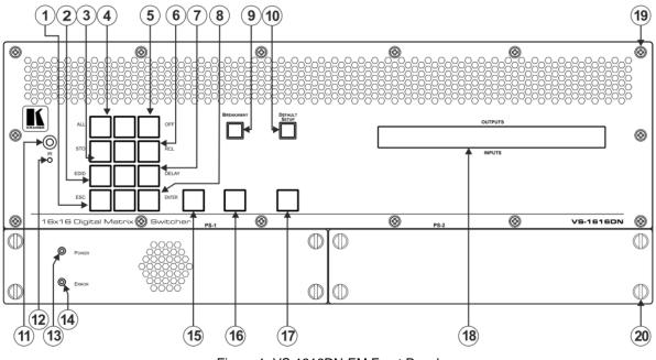
Figure 1: VS-1616DN-EM Front Panel
