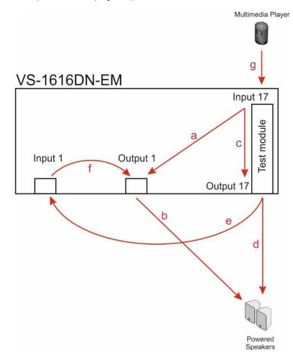
Figure 17: Signal Paths for Isolating Audio Problems
