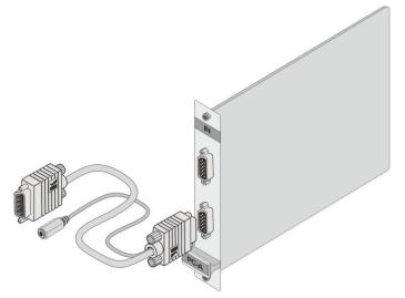
Figure 15: Accessing Audio over VGA
