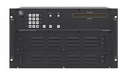
VS-3232DN-EM is a high-performance 4x4 to 32x32 4K@60Hz (4:2:0) modular matrix switcher chassis for AV signals. The unit is a multi-format digital switcher, populated from 4x4 to 32x32 in increments of four inputs and/or four outputs. The chassis includes optional dual, redundant power supplies, a control module and a test module that can monitor and test any input and output in the matrix. VS-3232DN-EM supports a wide variety of input and output cards for different AV signals
