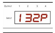
In this example: Input 1 is routed to output 1, input 3 is routed to output 2, input 2 is routed to output 3 and a pattern is routed to output 4.
