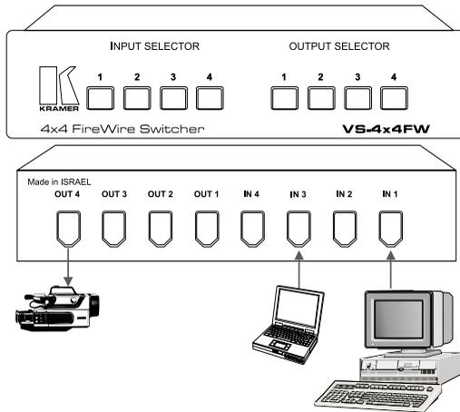
Figure 2: Connecting the VS-4x4FW 4x4 FireWire Switcher
