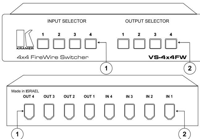
Figure 1: VS-4x4FW 4x4 FireWire Switcher
