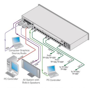
\* Note: The TP-133 transmitter can only be paired with a TP-134 receiver and the TP-125 transmitter can only be paired with a TP-126 receiver
