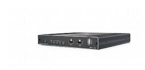
VW-4 is a 4-output video wall driver designed to quickly and easily configure and manage video walls. Use one VW-4 device to create any wall configuration with up to 4 displays, for example, a 2x2, 4x1, 1x4, 2x1, 3x1 video wall. Connect additional devices to create walls of any size and configuration of up to 64 displays. Configure a single or multiple device setup using the VW-4 app via Ethernet or RS-232, or quickly configure a basic setup using the local dip switches
