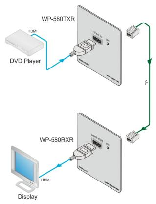
Figure 5: Connecting the WP-580Txr/WP-580Rxr Transmitter/Receiver Pair
