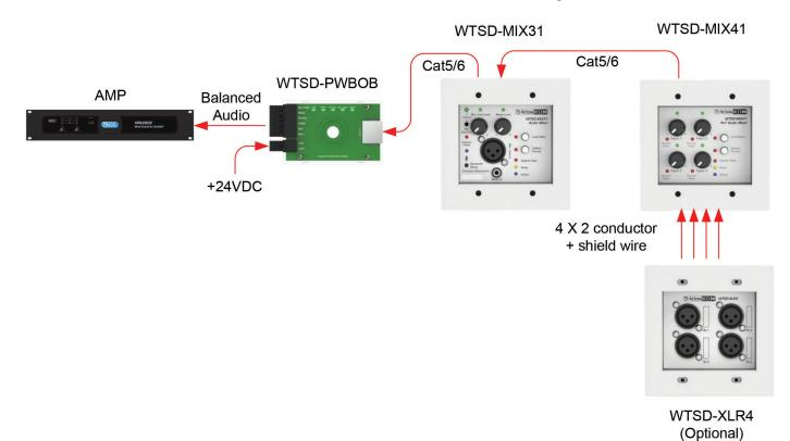
WTSD-MIX41 Cat5/6 WTSD-PWBOB **AMP** Balanced Audio +24VDC 4 X 2 conductor + shield wire INPUT OPTIONS NOTE: For Stereo RCA & 3.5mm Inputs Use ATLASIED AA-YSUM CABLE Input 2 Input 1 Input 4 Input 3
