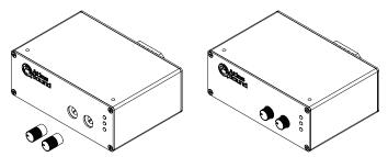
Security Cover Installation - Remove the knob from the panel and insert the cover.
