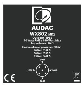
When the loudspeaker is connected to 70.7V facilities, the power indicated in the image on the previous page will be reduced to half the power, and when connected to 50V facilities, the power will be reduced to a guarter.
