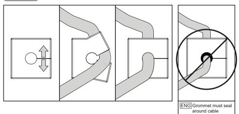
ENG Slide grommets into enclosure, aligning grooves of grommet with grooves in cable gland.
