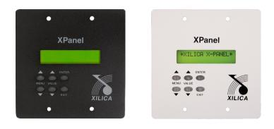
XPanel series are static IP remote controls, available in both black and white. XPanel controls allow the user to define the parameters controlled and the minimum and maximum values of the parameters range. Up to 32 XPanels can reside in one network. The front panel provides an LCD screen display, up/ down menu, up/down values, enter and exit buttons. The XPanel can be powered using PoE or an external power supply is included.
