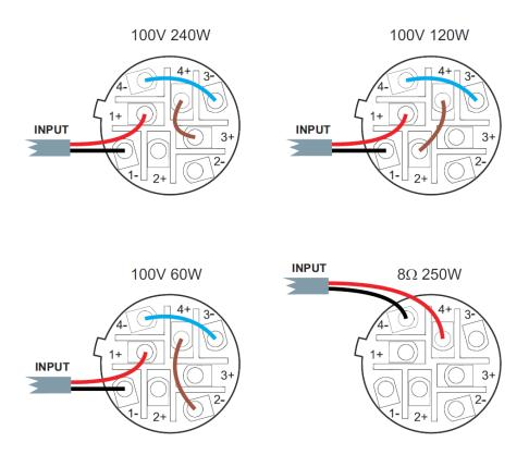
Figure 1: Speakon<sup>©</sup> connection diagram
