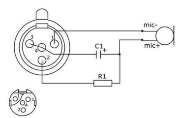
Pin 1: connected to the negative (-) pole of the microphone
