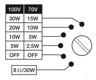
Figure 1: rear panel's power selector
